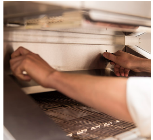
Adjustable infeed height: 45 - 85 mm.
